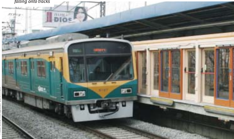
Train on metro line 1 approaching a station with protective door screens on the platforms to prevent passengers from falling onto tracks
